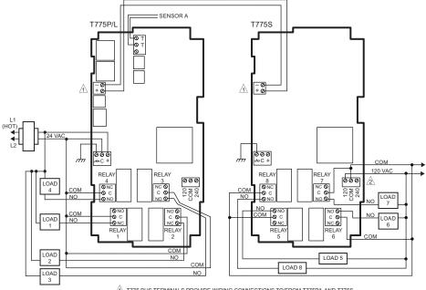
A T775 BUS TERMINALS PROVIDE WIRING CONNECTIONS TO/FROM T775P/L AND T775S
